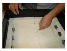
4. Remove the floor brick by placing a screwdriver tip between the floor bricks
