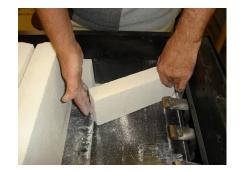
Slide one side of the back wall brick away from the back. Remove and set aside.
