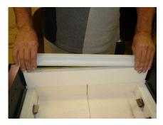
19. Reinstall marinite cover and tighten the screws on the back of the broiler.
