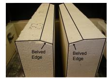
13. On the broiler floor stand the floor bricks on the flat edge with the beveled edges up and facing each other.
