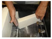
10. Vacuum the broiler floor to remove excess brick particles.
