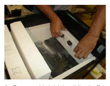
8. Remove side brick by sliding it off the Cobra heads and lift it out. Place aside.
