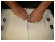
5. Pry up one side up enough to lift and remove the floor brick.
