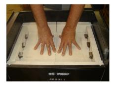
16. Press down with the same pressure in both hands until the bricks are flat on the floor of the broiler.
