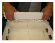
18. Replace the marinite bar by sliding down and into place.
