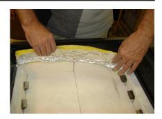
3. Lift out the insulation to expose the rear wall brick. Place aside.
